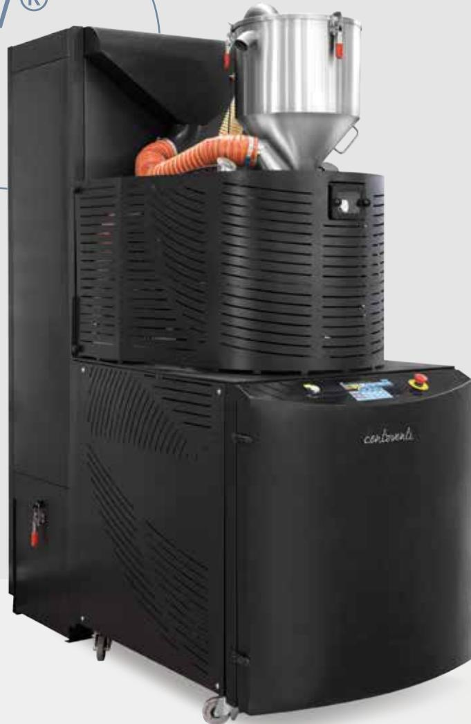
Suction system for filling hopper
